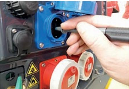
*Positive test result: measurement  $\leq 0.3$  ohm*
