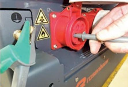
*Positive test result: measurement in each case min. 1 ohm*
