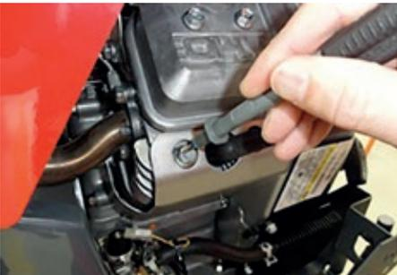
*Positive test result: measurement  $\leq 0.3$  ohm*
