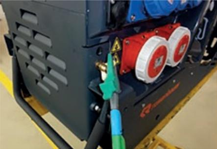
2. Measure contact resistance at the metal surfaces of the engine to the PE-contact:
