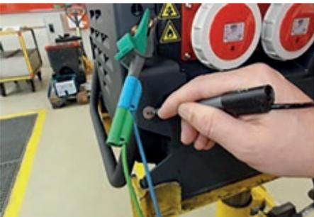
*Positive test result: measurement  $\leq 0.3$  ohm*
