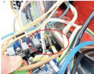
Reconnect the two ends of the potential equalization conductors:
